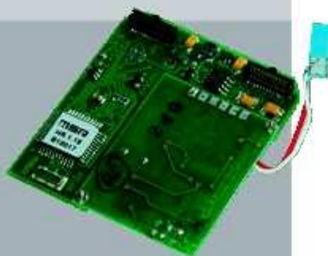
MSR 12 plug-in heart rate module HR
