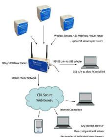
Fortunately, the RDL//1000 wireless sensor system from CDL was there to monitor everything. With its quick and easy setup and robust battery powered sensors it proved to be incredibly simple to keep an eye on everything. The system monitored combinations of ambient temperature and humidity and wood moisture levels, at intervals of 15 minutes, and sent the data to the CDL SmartHub via its own on-board GSM function once every hour.
