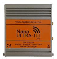
On board memory (for when communications are interrupted)
